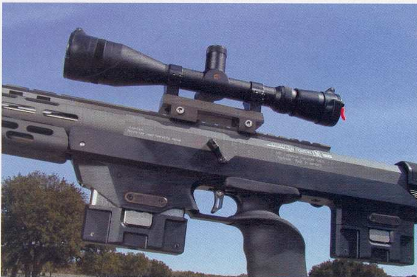
Left side view of receiver showing safety, dual magazines.
