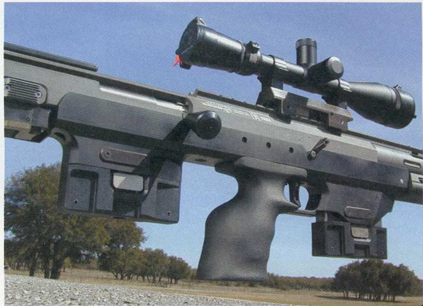
Right side of receiver showing bolt handle, dual magazines and safety. Small-elongated button at center left is the adjustment button for the cheek piece.
