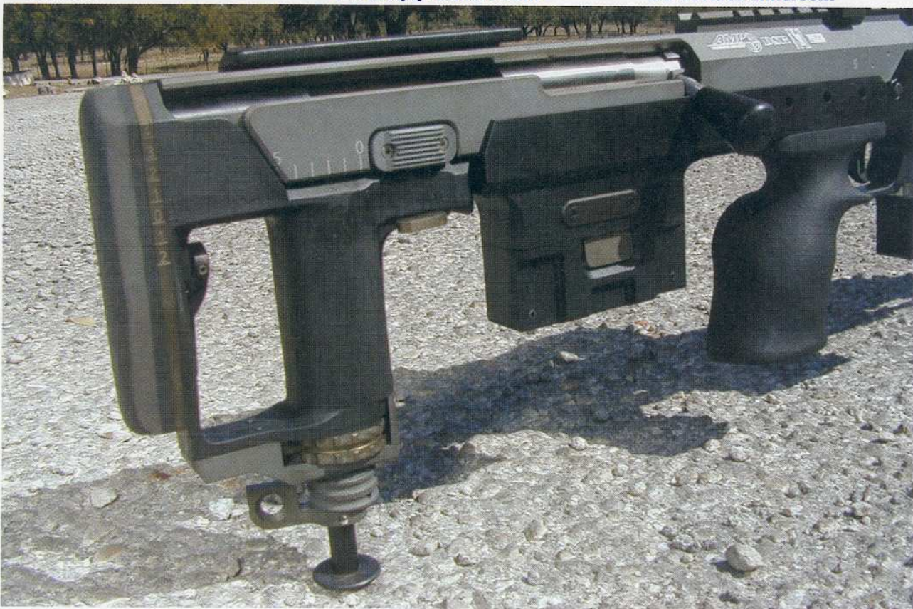
Showing rear of rifle with adjustable butt pad and monopod adjustment knobs. Above the monopod is the adjustable cheek piece.
