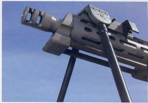
Muzzle brake of dual chamber design and suspension type adjustable bipod.
